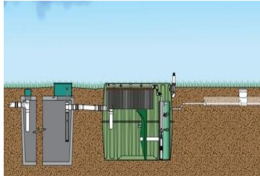
*ATTs are placed after a septic tank to utilize more efficient aerobic bacteria in the wastewater by introducing aeration (and oxygen) to the treatment process before sending it to a drainfield for final treatment and dispersal. (Image courtesy of Orenco Systems, Inc)*
